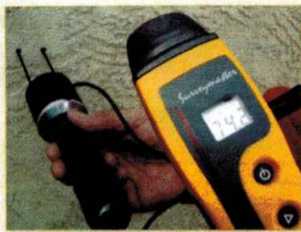
A moisture reading of 74.2 percent indicates a serious problem.
