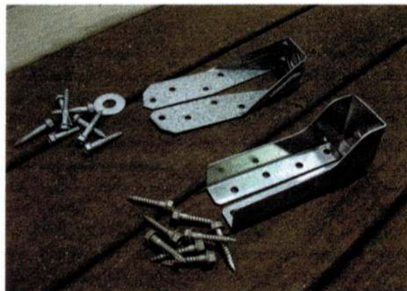
Figure 2. The two most common galvanized-steel lateral-load brackets are Simpson's DTT-2Z (top) and USP's DTB-TZ (bottom). Both are sold with a 1/2-inch washer and structural joist-attachment screws. You'll need a pair of brackets to make one connection, and will have to supply the threaded rod or bolt and nuts to join them together.
