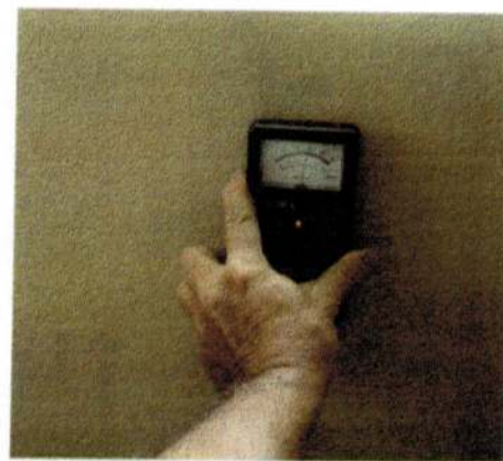
Photo 15: I typically measure moisture levels in walls below windows using a Tramex Moisture Encounter meter. I then compare the reading with a reading taken on the wall near the window. If I find elevated moisture levels below the windows, I know that there's likely to be concealed damage.
