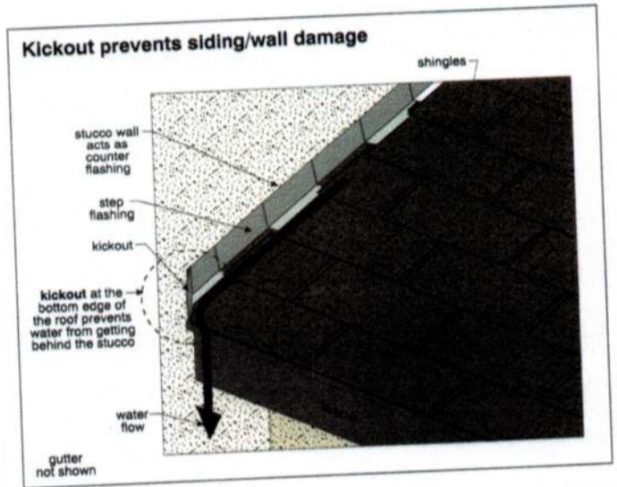
Kickout flashings prevent water from getting behind stucco at the bottom of adjacent roofs.
